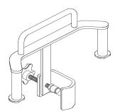
Always mount the tandem carrier (List# 12270-01) to the pole before attaching the pump(s) to the tandem carrier.
